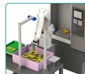
Picking from a large pallet (Fixed camera)
