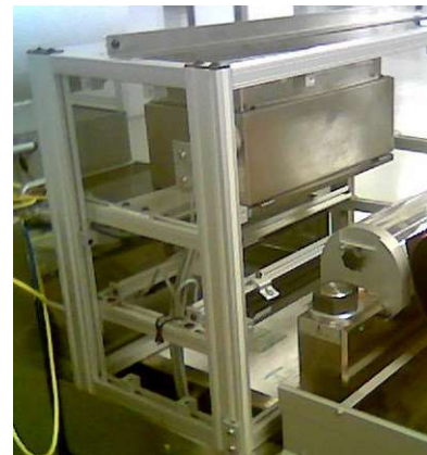
Label quality system installed over the web of a form, fill, and seal machine.
