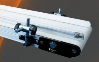
Adjustable side rails offer the ultimate in flexibility. Available guide heights are 1" (shown), 2", and 3". Standard guides may be adjusted approximately 3" vertically and horizontally. These guides are available with optional thumb screws (shown) for tool-less adjustments.
