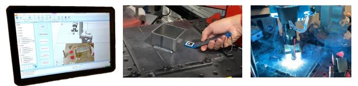
Our package combines AI, 3D Vision and Process Rules to enable non-experts to program robots code free. The robot is equipped with the sensor inputs and process knowledge it needs, so an operator can teach a task to the robot in the same way he would teach another human, just by pointing to where the process should be done and letting the robot figure out the details.
