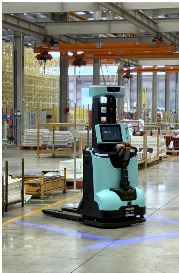
Our self-driving pallet jack is dual-mode: it can be used like a standard electric pallet jack and it can drive itself along preselected routes, freeing the operator for other tasks.
